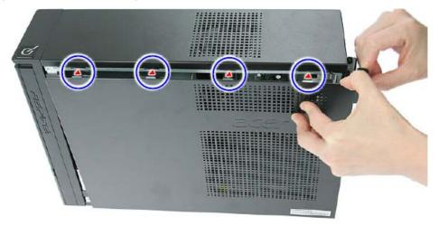
3. Push the side panel toward the front of the chassis until it is firmly closed.
